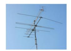
Mast head amplifier too close to the antenna
